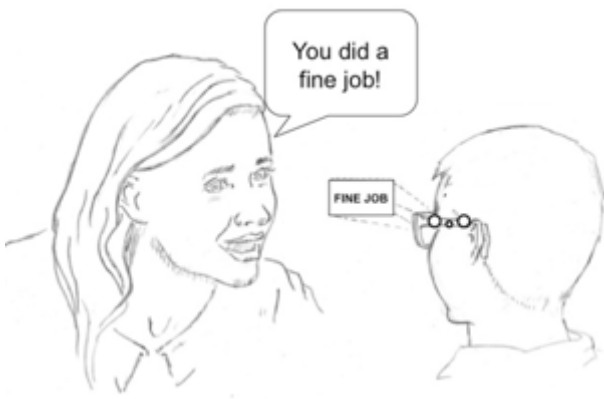
Figure 7. Schematic illustration of how a child with a HUD can read a transcription of what the mother is saying. the iPhone. Given our ASR implemented on the iPhone, we can perform the automatic speech recognition and transmit the resulting text to these eyeglasses.
